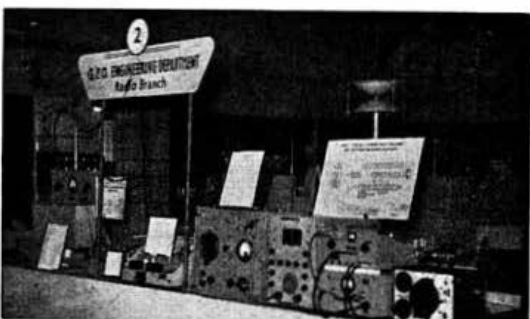
A corner of the G.P.O. Engineering Department Stand at the Amateur Radio Exhibition. In the foreground is Spectrum Measuring Equipment for use on frequencies in the 2,300-2,450 Mc/s. amateur band.
